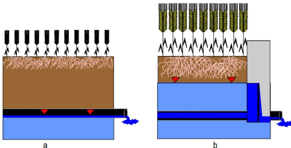
*Fig. 2. Conventional (a) and controlled (b) drainage systems*
