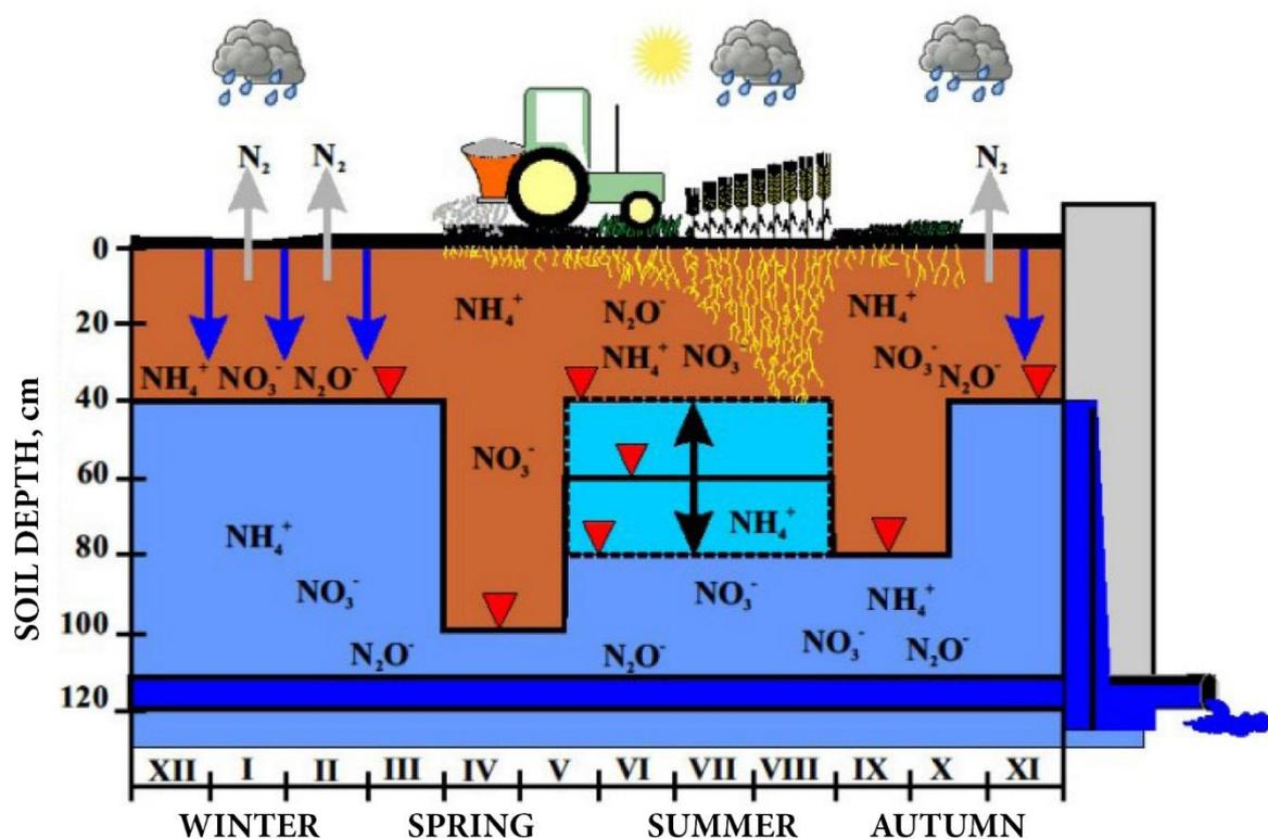
*Scheme of water level-controlled drainage system*
