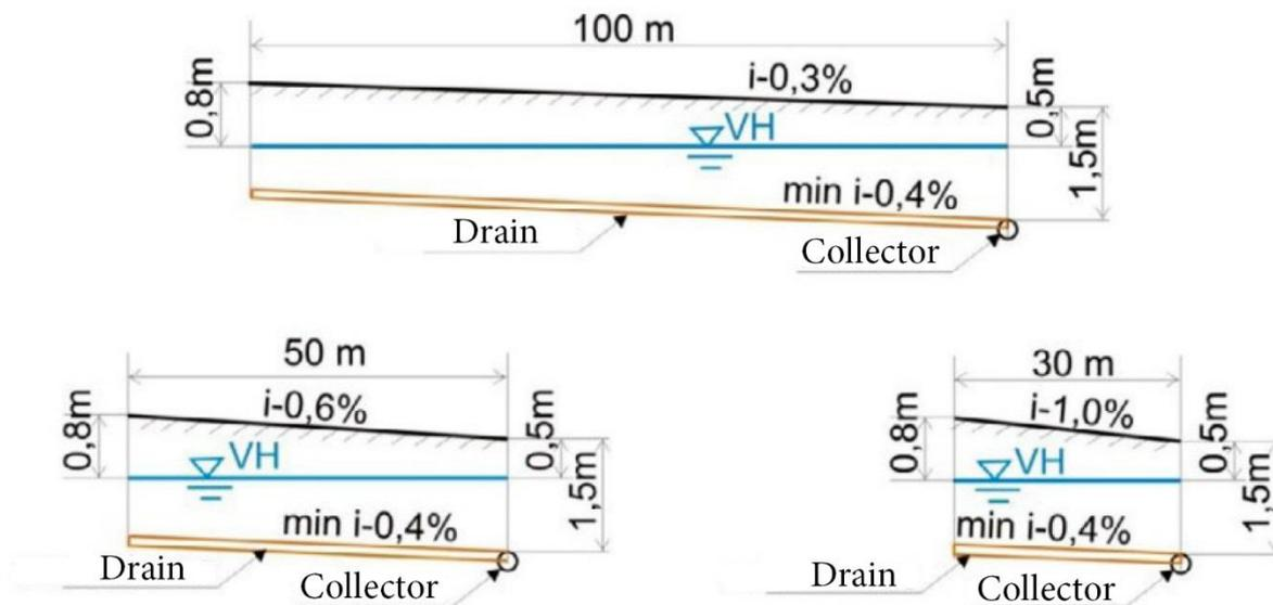
*Fig. 1. Influence of land surface slope on drainage head length*
